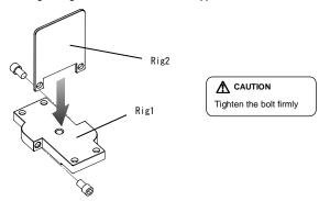
2. Mount each camera on the base assembled in step1 and secure them with the supplied bolts
