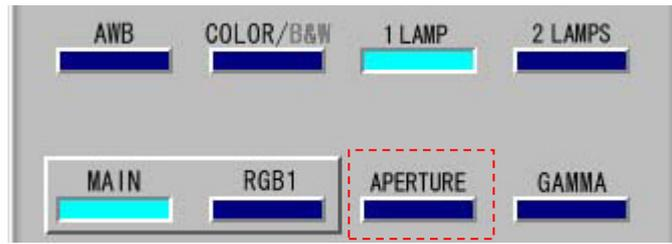
Click the [APERTURE] button to switch ON/OFF the image enhancer (countor) of the main unit.
